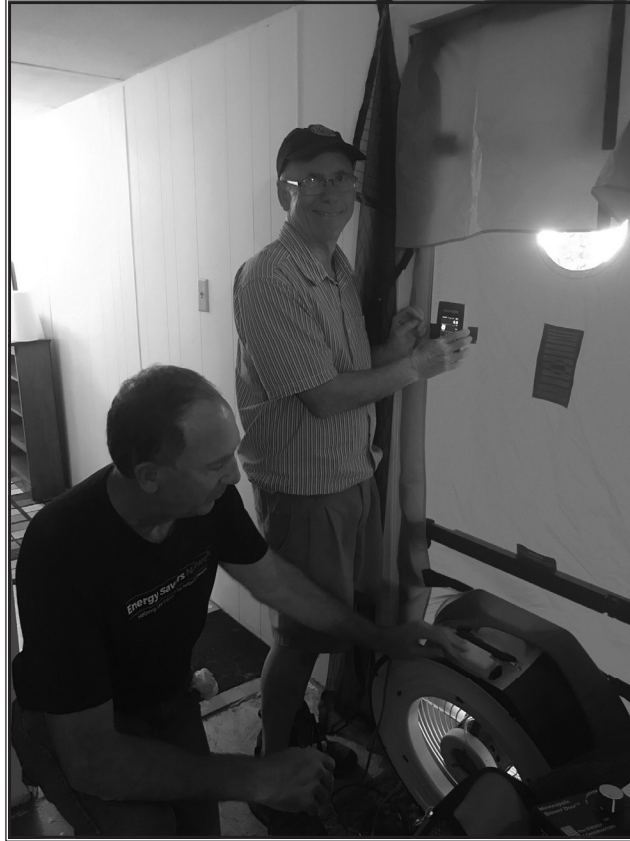
Brad and volunteer Joe Wombwell using blower door to test for air leaks on mobile home.
